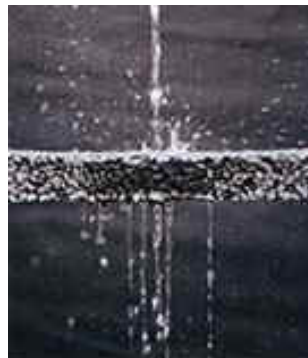
Figure 4.3 Cross-Section of Pervious Concrete
